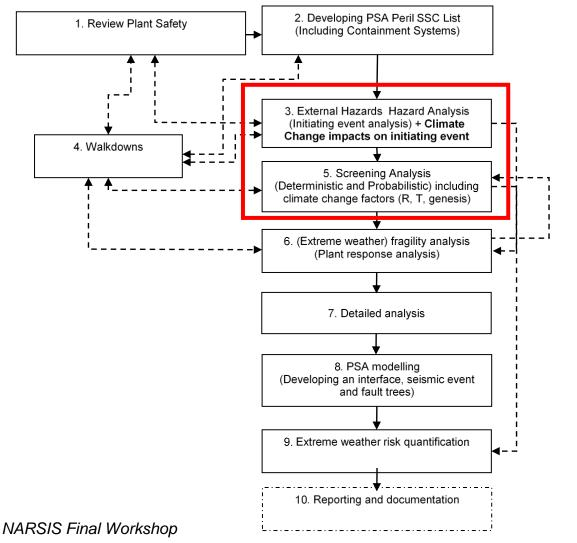
Flow chart for extended Level 2 PSA showing the proposed location of the multi-hazard framework component
