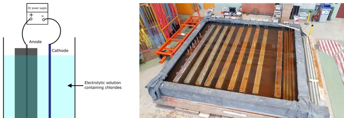
Figure 2. Accelerated corrosion technique: set-up principle (left) and CEA beams under corrosion (right).
